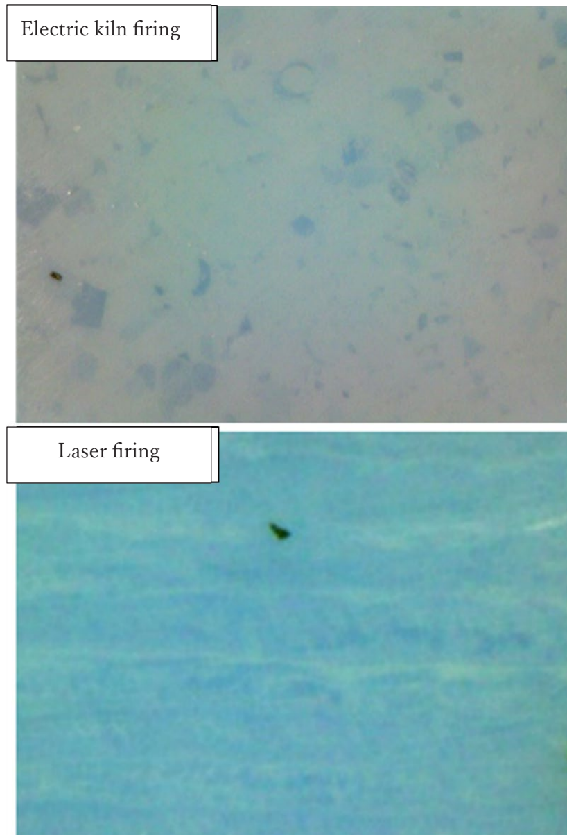
Fig. 12: Firing Results of Blue Glaze — a) Electric Kiln Firing, b) Laser Firing
