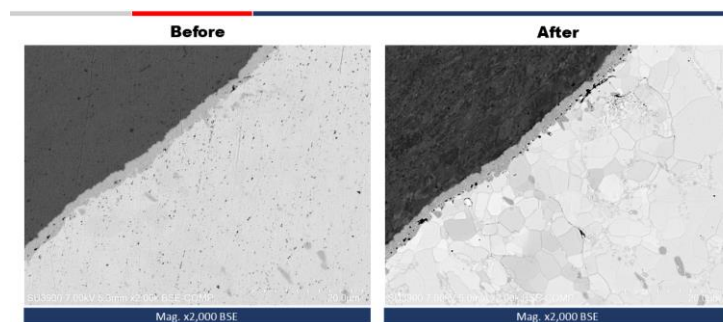
SEM condition : Model SU3900, Accelerating voltage 7 kV, BSE signal Flat milling condition : Accelerating voltage 3 kV, Time 7 min.
